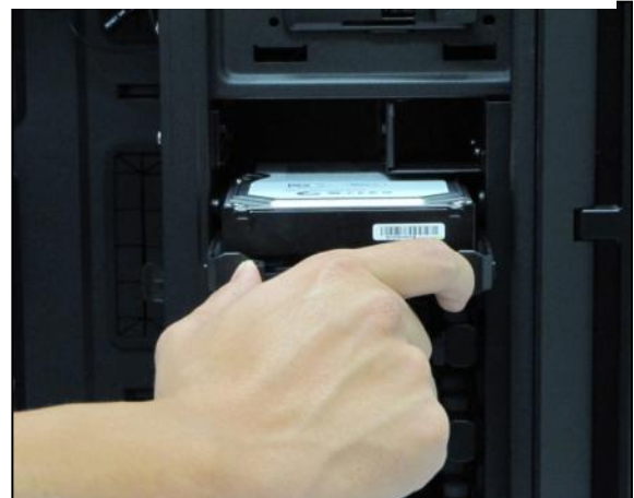
Pinch the ends of the tray and insert your drive until it clicks.
