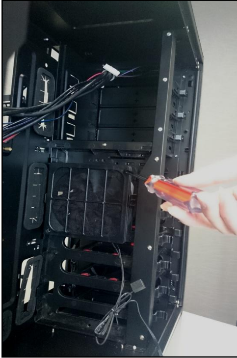
Secure an intake fan into place by aligning it with the pegs that correspond with the fan screw holes.
