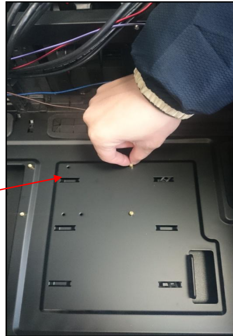
Install the motherboard standoffs by aligning the motherboard with the standoff holes.
