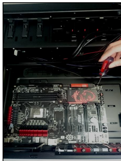
Use the provided motherboard mounting screws to secure your motherboard into the standoffs.
